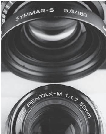
**Figure 3.3** Engraving around lenses here shows (top) name of lens; maximum aperture  $f/5.6$  and focal length 180 mm and (bottom) name,  $f/1.7$  maximum aperture, 50 mm focal length
